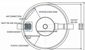
Note: Drawing of WWTP for backfill or concreeting. Assembly make according to the Instruction for installation.
